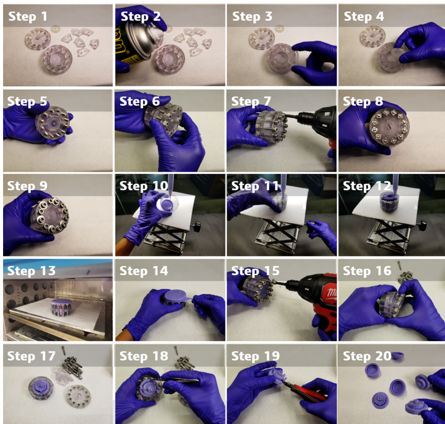
Figure S8: The amplifier's gate is made using fabrication approaches familiar to the field of soft robotics including injection-molding with elastomers. 3
