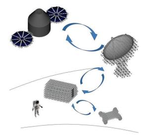
Figure.12. POTENTIAL APPLICATIONS OF OUR PROPOSED CHAIN DESIGN IN SPACE EXPLORATION. *NOTE*: THE FRAMES OF THE ANTENNA AND SOLAR PANEL ARE ALL FOLDED BY THE SAME CHAIN WITH 1554 LINKS.
