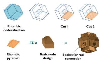
Figure. 3. THE FORMATION OF THE BASIC NODE GEOMETRY. TOP ROW: A SMALLER RHOMBIC DODECOHEDRON IS FIRST FIT INTO THE CENTER OF THE BUSIES CONNECTION JOINT. BOTTOM ROW: AFTER A SERIES OF CUTTING PROCESS, THE RHOMBIC PYRAMID SHAPE IS SELECTED TO FORM BASIC GEOMETRY OF NODE DESIGN.
