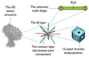
Figure. 2. SCHEMATIC DRAWING SHOWING THE DIFFERENT COMPONENTS AT THE BUSIEST CONNECTION JOINT INSIDE A LARGE THREE-DIMENSIONAL LATTICE STRUCTURE (AN ANTENNA FRAME).
