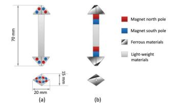
Figure. 5. TWO DIFFERENT TYPES OF MAGNETIC COUPLING USED IN OUR PROTOTYPE (a) TYPE-I – EMBEDDING PAIRED MAGNETS DIRECTLY AT THE CONTACTING SITES. (b) TYPE-II – TRANSMITTING MAGNETIC FORCES THROUGH THE NODE MADE OF FERROUS MATERIALS. *NOTE*: THE CENTRAL HOLE IS FOR ANCHORING CONNECTING STRINGS.
