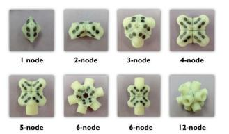
Figure. 6. POSSIBLE CONNECTION JOINTS SUPPORTED BY TYPE-I COUPLING METHOD. *NOTE*: EXCEPT FOR THE START AND THE END, ALL THE OTHER CONNECTION JOINTS HAVE EVEN NUMBER OF NODES INSIDE ANY FOLDED LATTICE STRUCTURE. RODS WERE REMOVED FOR BETTER VISIBILITY OF THE NODES.
