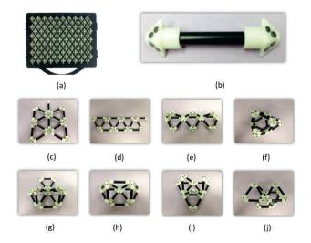
Figure. 8. The PROTOTYPING PROCESS OF NODES VIA 3D PRINTING. (a) A TRAY OF 110 3D-PRINTED NODES. (b) EXAMPLE OF A SEPARATE LINK. (c)–(j) VARIATIONS OF 2D AND 3D STRUCTURES FOLDED BY A 14-LINK CHAIN.
