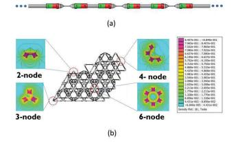
Figure. 7. 2D SIMULATION OF THE MAGETIC FIELDS BY USING TYPE-II COUPLING METHOD. (a) ALTERNATING THE POLES AT THE TWO ENDS OF EACH ROD. (b) 2D SIMULATION OF THE MAGNETIC FIELDS AT DIFFERENT CONNECTION JOINTS IN A 3D RECONFIGURABLE LATTICE STRUCTURE.
