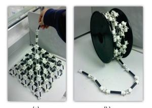
(a) (b) Figure. 1. PICTURES OF OUR PROOF-OF-CONCEPT DESIGN. (a) 293 LINKS ARE USED IN THE FOLDING OF THE PYRAMID SHAPE. (b) A SPOOL OF THE MODULAR CHAIN.
