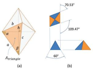
Figure. 4. THE IMPORTANT DIMENSIONS OF OUR NODE DESIGN. (a) THE RHOMBIC PYRAMID WITH FOUR SYMMETRICALLY IDENTICAL FACES. (b) SCHEMATIC DRAWING OF THE NODE DESIGN SHOWING THE CRITICAL ASSEMBLY ANGLES.
